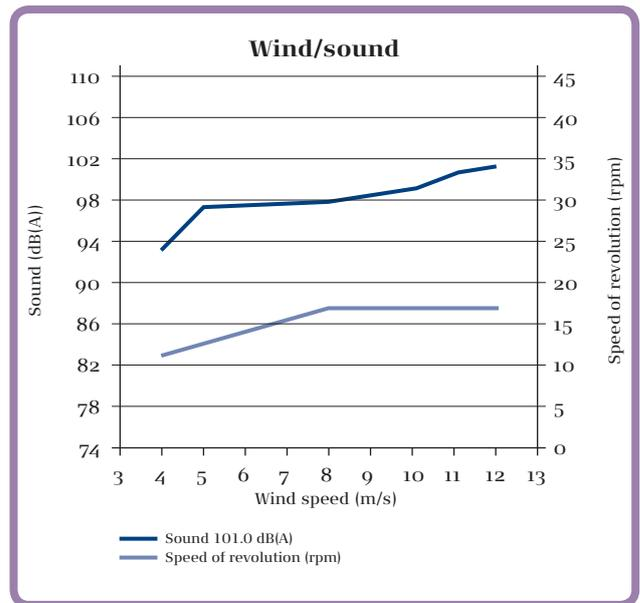
The sound output level can be adjusted by varying the revolution speed of the turbine as illustrated in the figure above. It clearly shows the sound level advantages of lower speeds of revolution because the sound level is approximately 7 dB(A) lower at 4 m/s than at 8 m/s. For other sound levels, the benefit can be as much as 10 dB(A). Please note that a decrease of 3 dB(A) represents a halving of the sound level.
